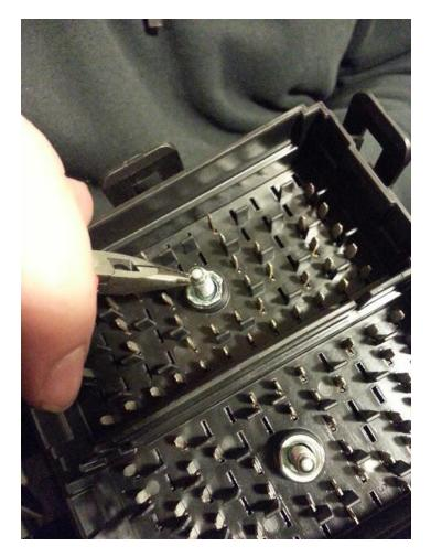
3. When un-swedged enough, knock the bolts through the box so that it can be disassembled. I messed up the bolts so badly (bad needle nose pliers) during the un-swedging that I decided to cut the metal sleeves surrounding the bolts (see picture) so that they don't interfere. The sleeves are not needed as their only purpose is to keep you from opening the fusebox. When the box is in the car, it is held in place by the four bolts and the four block modules.
