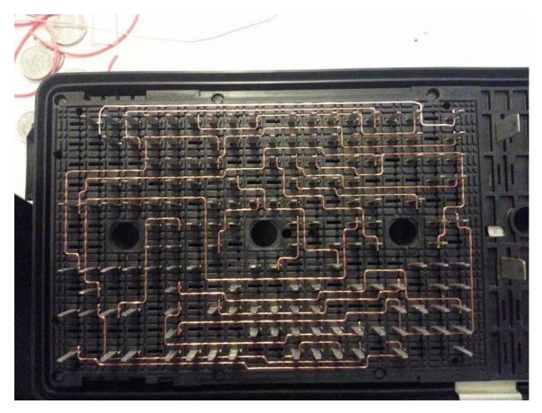
**Put everything back together and drive after dark!** When putting the fusebox back together, simply align the four block modules and place the box on top of them (without the bolts in place). Then see through the bolt holes so that you make sure that they are centered. Enter the bolts and screw in place each of the modules till each bolt is tightened. Check visually afterwards if all the blocks are in place.
