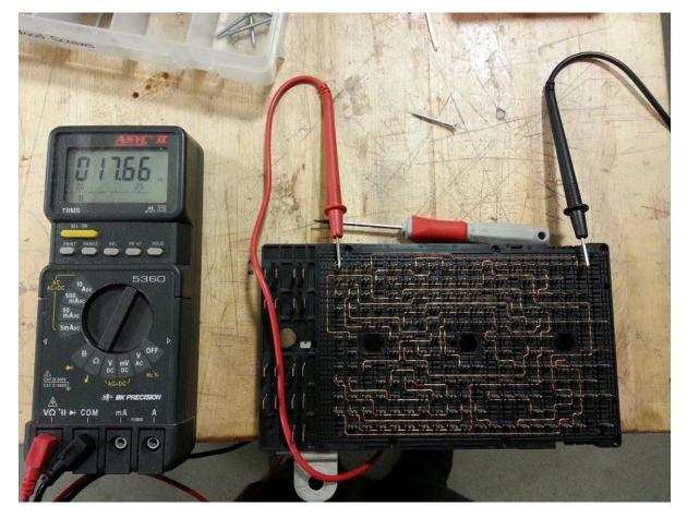
3. Replace the wire. As Tom suggested, I added a backup wire on the other side as well. So in case the wire breaks again there is a backup on the other side. I also removed some of the plastic guiding with a razor so that the copper wire can have nicer bends.
